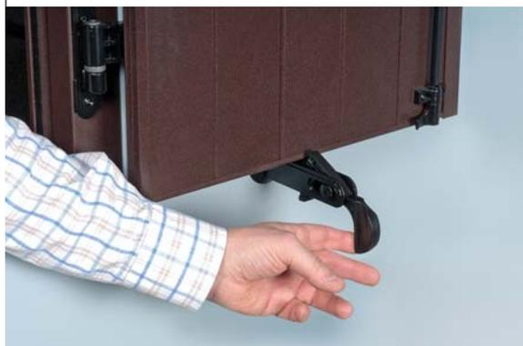
By lifting the stopping bow this is armed and the wall catch keeps open until the sash, when opening or closing, passes over it and unblocks it thus restoring the original position.
