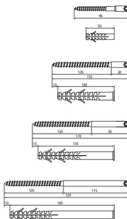
The supporting pin, available in 4 different lengths, is compatible with every kind of wall, both traditional and insulated.
