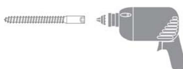
Thanks to the hexagonal impression on the head, the pin can be applied with a traditional screw before fixing the shutter stopper to it by using a threaded dowel.
